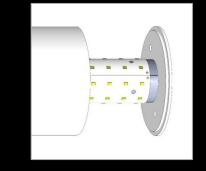
**90 cri** flexible planar LED lighting sheet wrapped around extruded aluminum core provides totally even luminance
